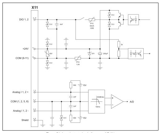
Figure 74: Input/output circuit diagram - AC131
