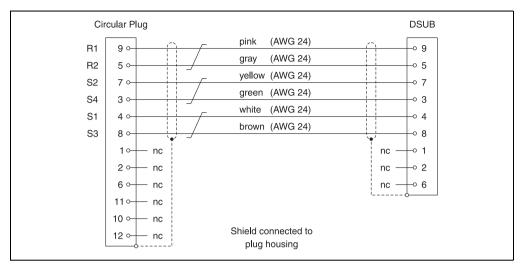
Figure 82: Cable schematic for resolver cables
