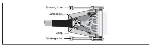
Figure 55: Cable shielding in DSUB housing
