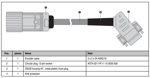
Table 183: Resolver cable construction
