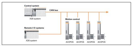
Figure 8: ACOPOS in a CAN bus network
