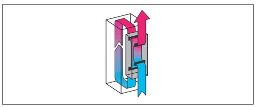
Figure 37: Function diagram of air/air heat exchangers
