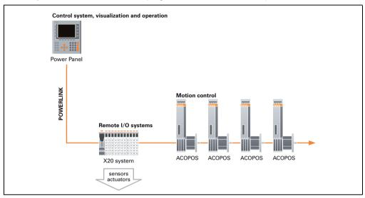
Figure 6: Compact, modular motion control applications
