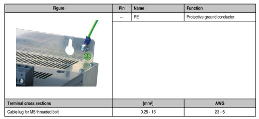
Table 149: Protective ground conductor (PE) ACOPOS 1180, 1320
