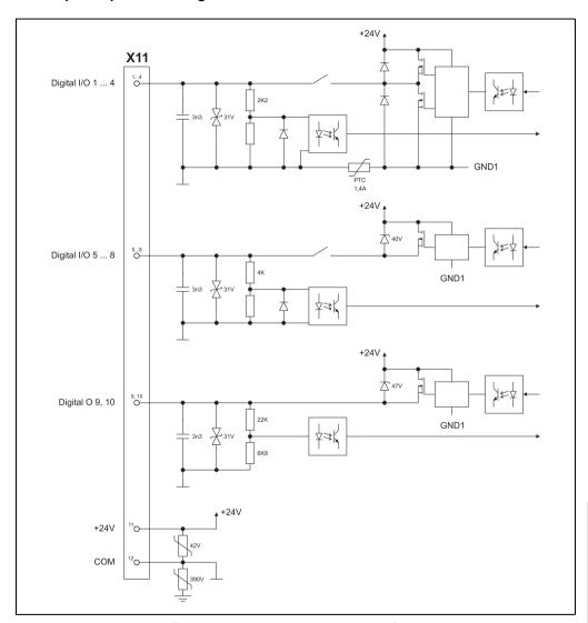
Figure 73: Input/output circuit diagram - AC130
