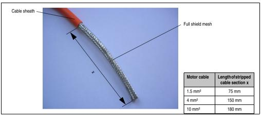
Figure 20: Stripped cable end
