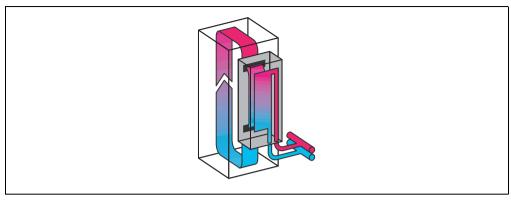
Figure 38: Function diagram of air/water heat exchangers
