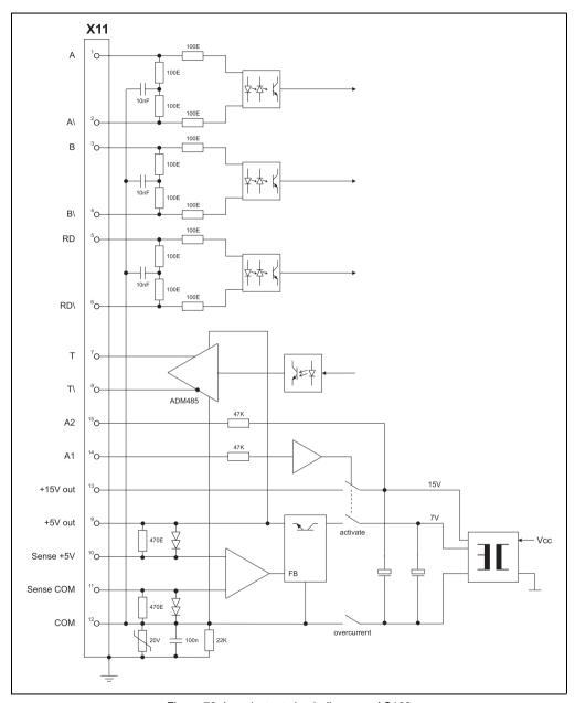
Figure 72: Input/output circuit diagram - AC123
