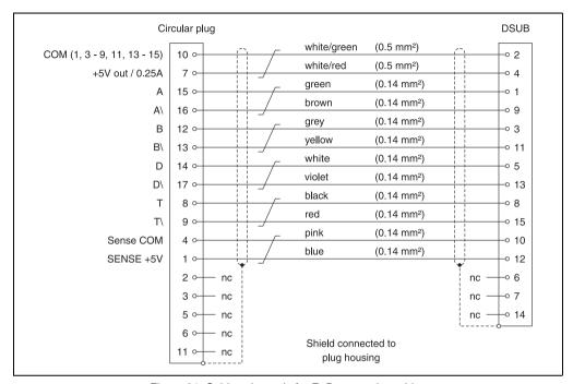
Figure 81: Cable schematic for EnDat encoder cables
