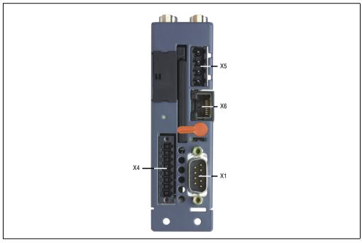
Figure 78: Overview of AC141 connections (view from below)
