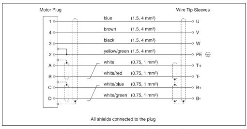
Figure 79: Cable schematic for motor cables 8CMxxx.12-1, 8CMxxx.12-3
