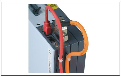
Figure 57: Connecting cables to plug-in modules
