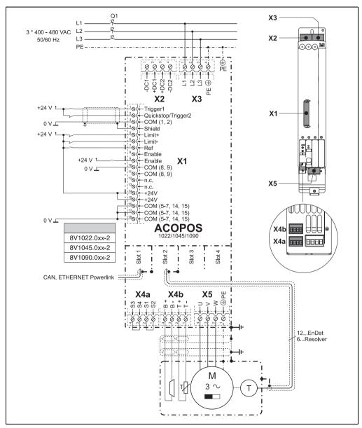
Figure 60: Overview of pin assignments ACOPOS 1022, 1045, 1090
