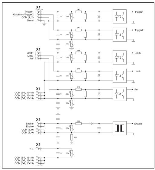
Figure 65: Input/output circuit diagram - ACOPOS 1640, 128M
