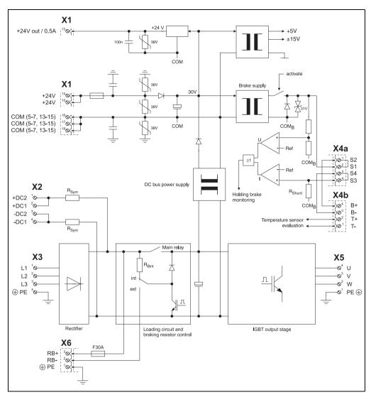
Figure 65: Input/output circuit diagram - ACOPOS 1640, 128M (cont.)
