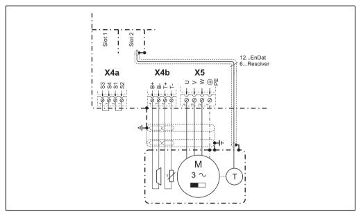
Figure 45: ACOPOS X4/X5 circuit diagram, motor connection
