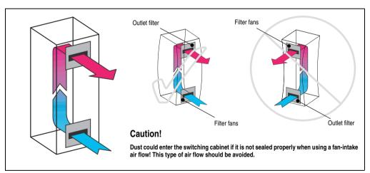
Figure 36: Function diagram of filter fans
