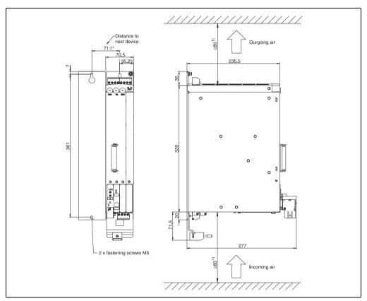
Figure 28: Dimensional diagram and installation dimensions for ACOPOS 1022, 1045, 1090
