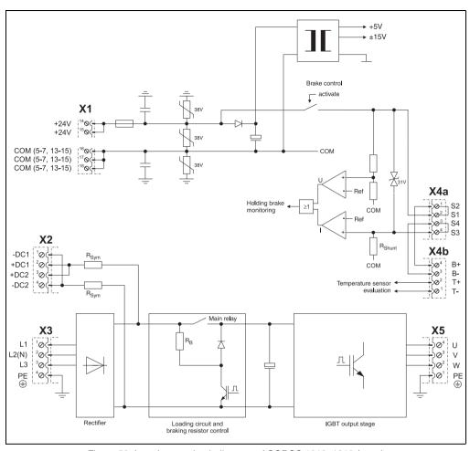
Figure 59: Input/output circuit diagram - ACOPOS 1010, 1016 (cont.)
