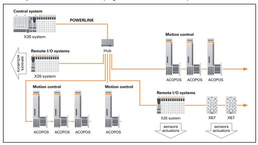
Figure 7: Extensive, modular motion control applications with up to 253 axes
