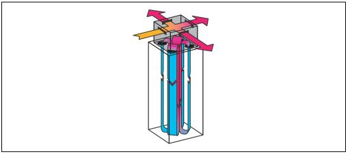
Figure 39: Placing a cooling aggregate on top of the switching cabinet
