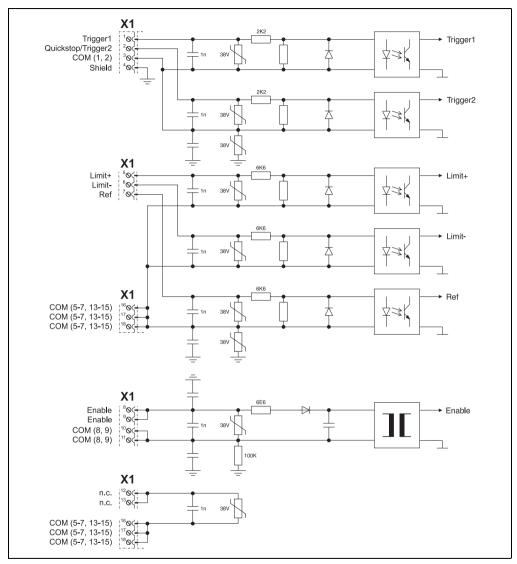
Figure 61: Input/output circuit diagram - ACOPOS 1022, 1045, 1090
