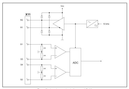
Figure 71: Input/output circuit diagram - AC122
