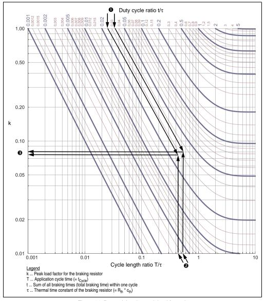
Figure 51: Determining the peak load factor k
