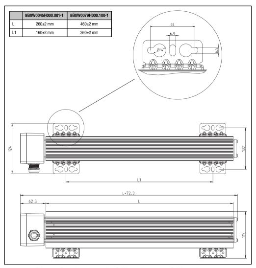
Figure 32: Dimension diagram for 8B0W0045H000.001-1, 8B0W0079H000.001-1
