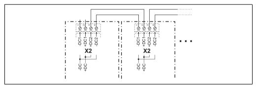
Figure 43: ACOPOS X2 circuit diagram, DC bus connections
