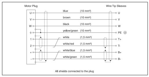
Figure 80: Cable schematic for motor cables 8CMxxx.12-5
