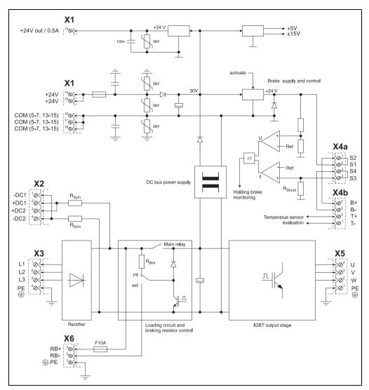
Figure 63: Input/output circuit diagram - ACOPOS 1180, 1320 (cont.)
