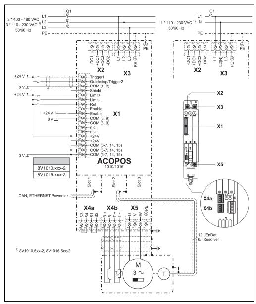
Figure 58: Overview of pin assignments ACOPOS 1010, 1016
