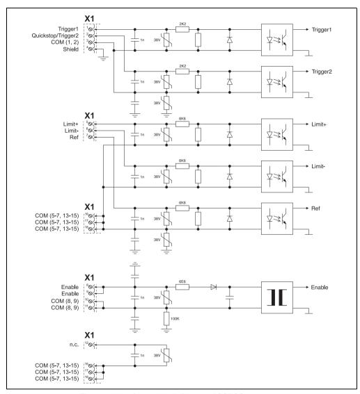
Figure 63: Input/output circuit diagram - ACOPOS 1180, 1320
