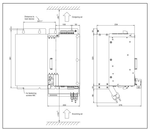
Figure 29: Dimensional diagram and installation dimensions for ACOPOS 1180, 1320
