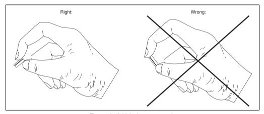
Figure 17: Hold the battery correctly
