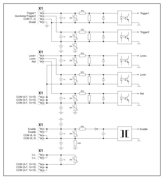
Figure 59: Input/output circuit diagram - ACOPOS 1010, 1016
