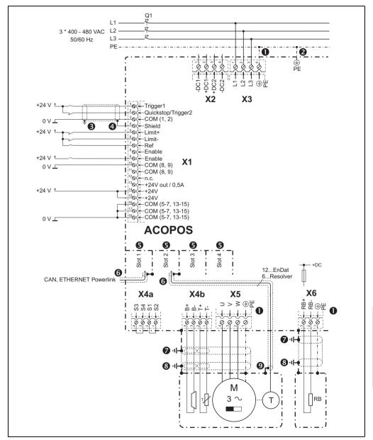
Figure 54: Connection diagram for ground and shield connections
