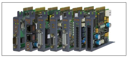
Figure 2: Plug-in modules allow optimized, application-specific configuration of ACOPOS servo drives
