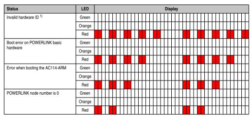
Table 8: Error status with reference to the POWERLINK V2 plug-in module AC114
