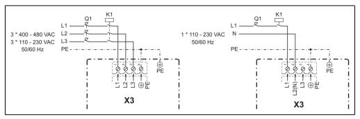
Figure 41: Circuit diagram for ACOPOS X3, individual power mains connection
