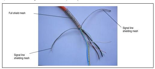
Figure 23: Cable end without stranding elements
