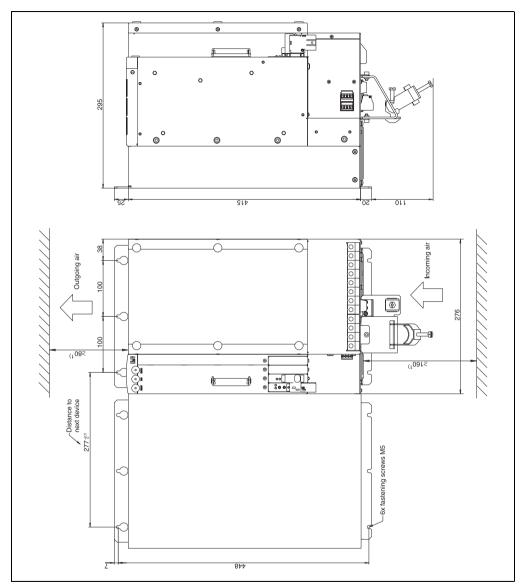
Figure 30: Dimensional diagram and installation dimensions for ACOPOS 1640
