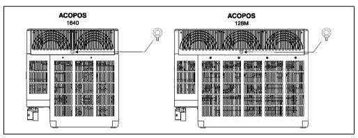
Figure 19: Attaching the eye bolt contained in the delivery to ACOPOS 1640, 128M drives
