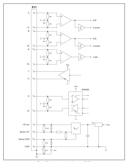
Figure 69: Input/output circuit diagram - AC120
