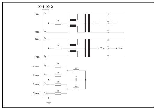
Figure 68: Input/output circuit diagram - AC114
