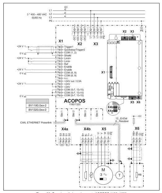
Figure 62: Overview of pin assignments ACOPOS 1180, 1320
