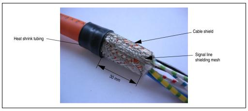
Figure 25: Attaching the shielding mesh
