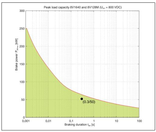
Figure 50: Peak load capacity - 8V1640 / 8V128M
