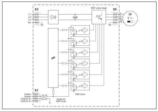
Figure 1: Block diagram of secure pulse disabling
