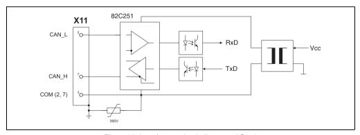
Figure 67: Input/output circuit diagram - AC110
