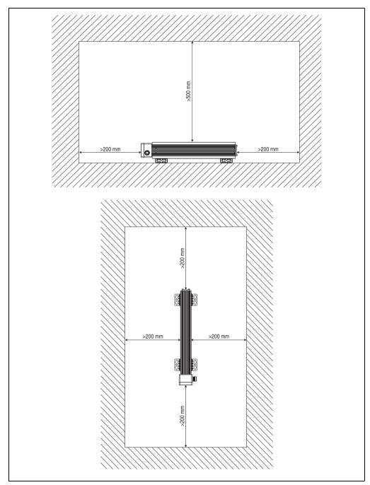
Figure 33: Installation dimensions - 8B0W external braking resistors
