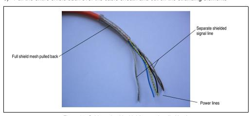
Figure 21: Cable ends with shielding mesh pulled back
