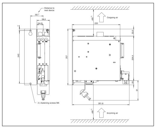
Figure 27: Dimensional diagram and installation dimensions for ACOPOS 1010, 1016
