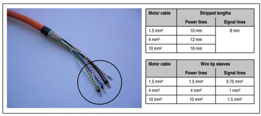
Figure 26: Wire ends with wire tip sleeves
