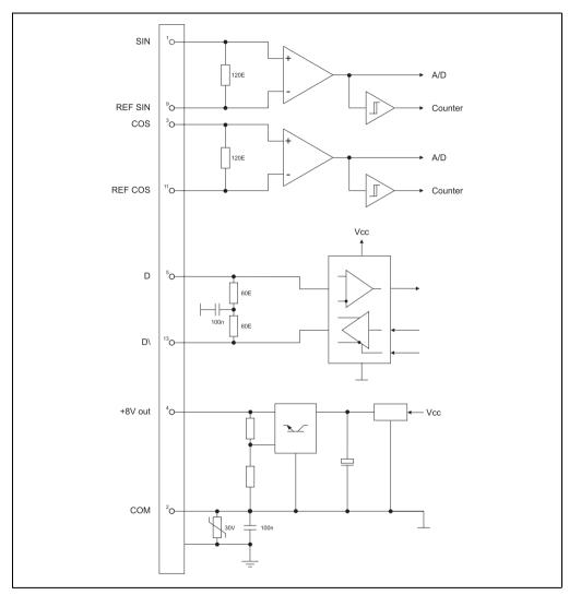
Figure 70: Input/output circuit diagram - AC121
