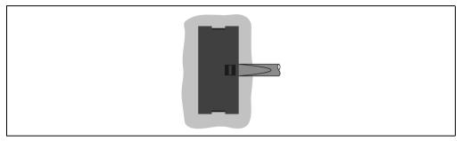
Figure 13: Remove the cover for the lithium battery
