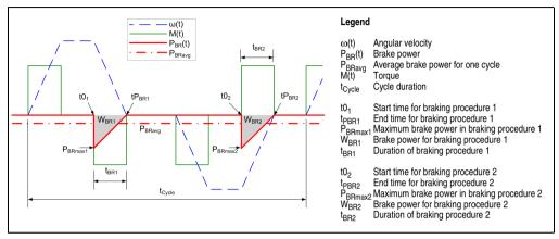
Figure 47: Movement and load profile for one axis in a sample application
