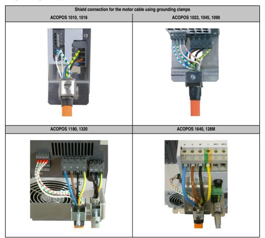
Table 121: Grounding of the motor cable on the ACOPOS servo drive
