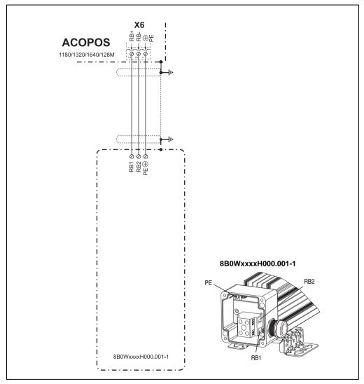
Figure 66: Overview of pin assignments - 8B0W
