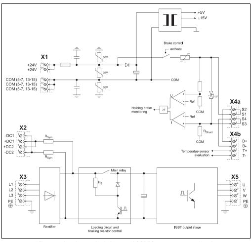
Figure 61: Input/output circuit diagram - ACOPOS 1022, 1045, 1090 (cont.)
