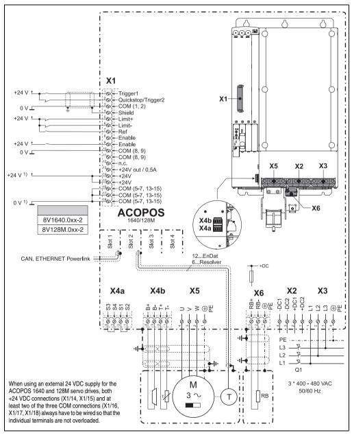
Figure 64: Overview of pin assignments ACOPOS 1640, 128M
