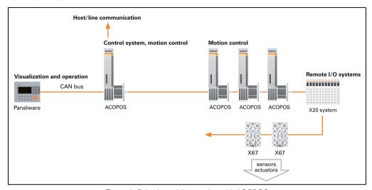
Figure 9: Drive-based Automation with ACOPOS
