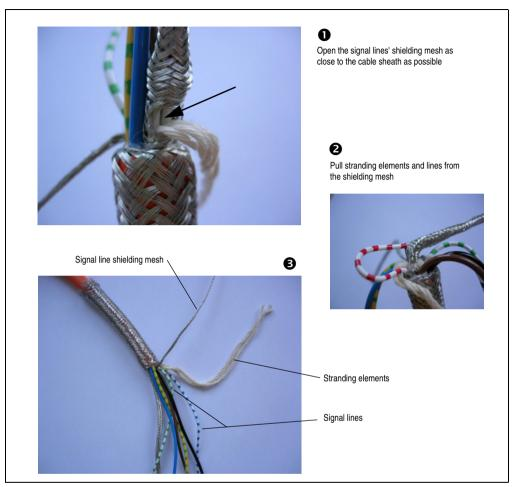
Figure 22: Pulling out the separately shielded signal lines
