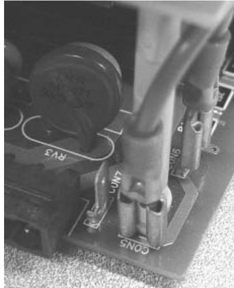
Grounded Input Power Configuration (Factory Default) CON5 Jumpered to CON6
