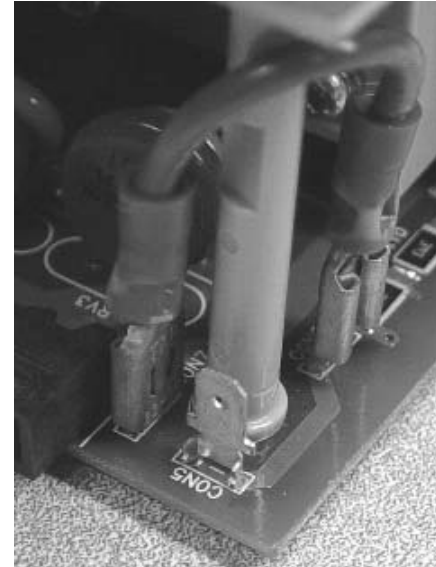
Ungrounded Input Power Configuration (Field Selected) CON6 Jumpered to CON7
